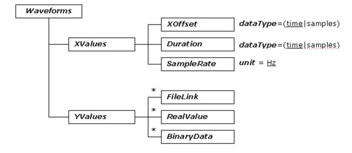
Figure 5 The tree diagram of ecgML: *Waveforms* element
