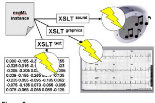
Figure 8 Dynamic transformation of ecgML data
