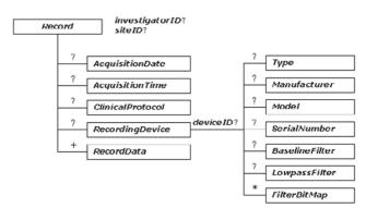
Figure 2 The tree diagram of ecgML: Record element
