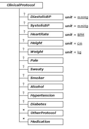
Figure 3 The tree diagram of ecgML: ClinicalProtocol element
